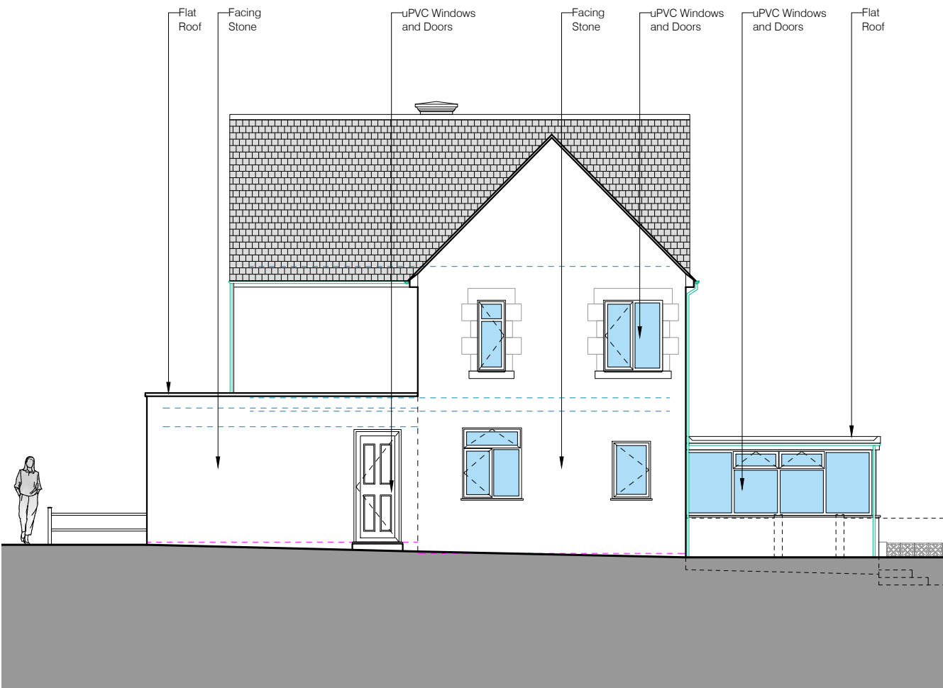
FRONT ELEVATION AS EXISTING SCALE - 1:100@A1
