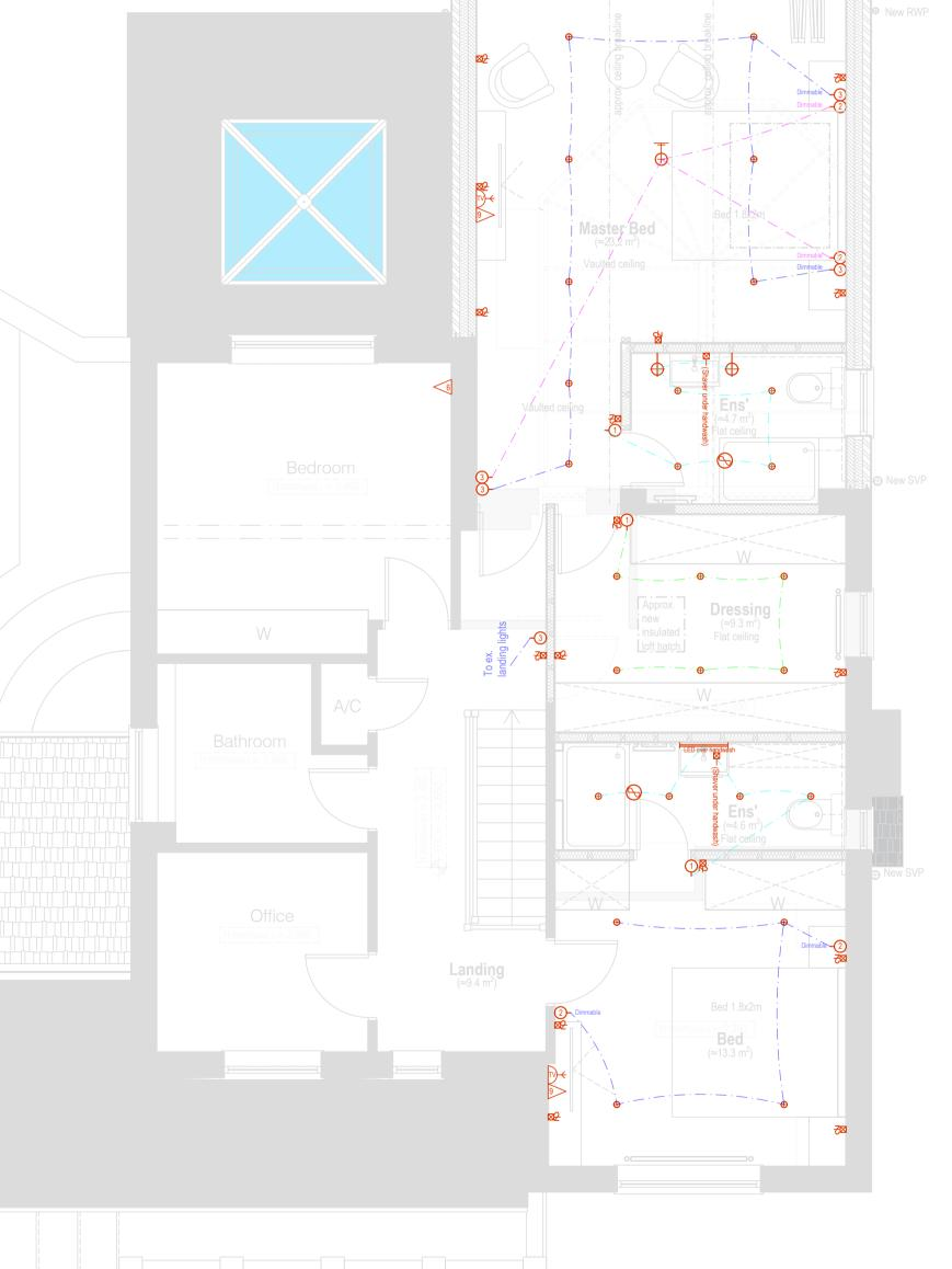
Electrical key: Down light/ Spot light - Wall Light - Pendant Light - LED batten
