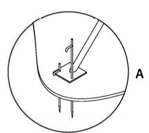
Heras panels (or equivalent) fixed in position as indicated with ground pins
